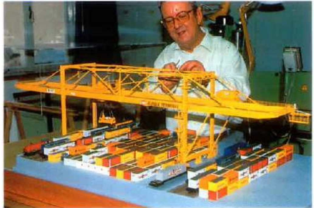
Werner Mischler with his 1:87 scale all-metal model of the 110-metre gantry crane in Basel harbour. Some 85% of all the joints were made by bonding with Araldite.
